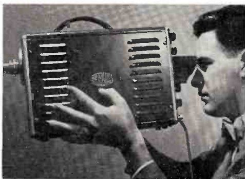
AN 18-POUND portable TV camera designed to replace a standard 350-lb. setup was shown by Allen B. DuMont Labs. at the IRE convention. Called the Tel-Eye, the camera will plug into a standard wall socket. It is 14 in. long, 9¾ in. high and 4¾ in. wide. DuMont sets the price at $2,850.
